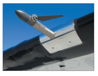
That's the angle-of-attack vane on the wing's leading edge of a PC-12NG.
