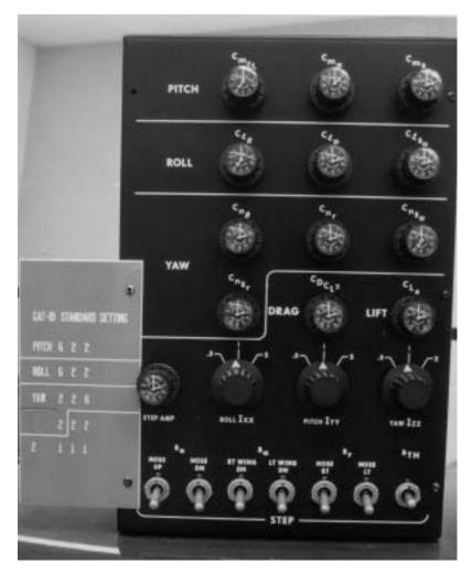
Figure 5. The GAT-IVS variable stability control panel.
