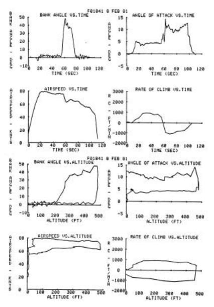
Figure 11b. Graphic output of the flight parameters from a successful test flight.
