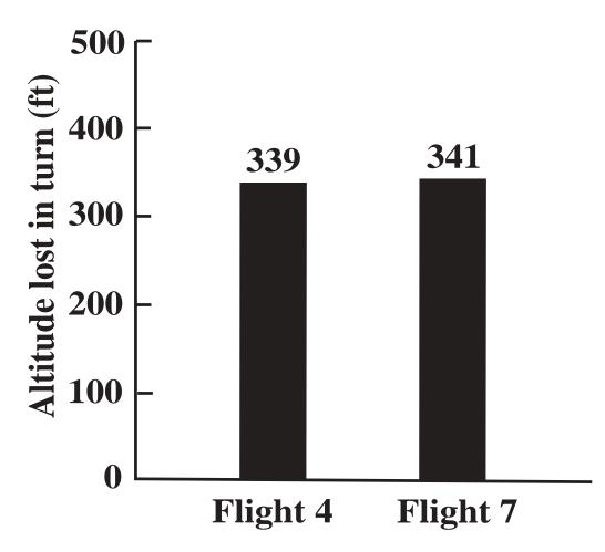
Figure 17. A comparison of the altitude lost in a 180° turn for flights 4 and 7.
