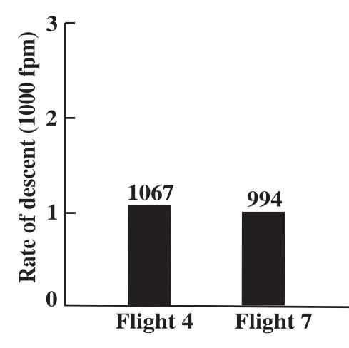
Figure 18. A comparison of the rate of descent upon turn completion for flights 4 and 7.
