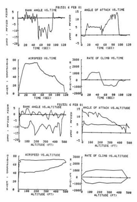
Figure 12b. Graphic output of the flight parameters from of an unsuccessful test flight.
