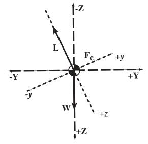
**Figure 1.** Forces in the *yz* plane acting on an aircraft in a steady state gliding turn.
