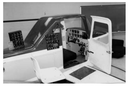
Figure 8. The GAT-IVS control panels, cockpit and instrument panel.
