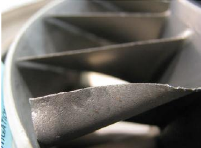
First Stage rotor icing damage
