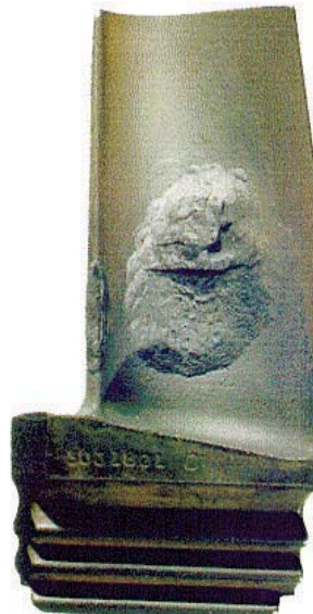
Stage 3 -Severe sulphidation
