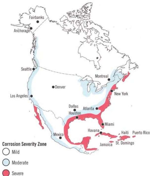
North American Corrosion Severity Map, extracted from FAA Advisory Circular 43-4A,
