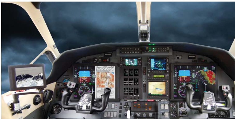
The IS&S integrated cockpit flat panel display system installed on a PC-12 shows primary flight data and an approach chart. The 5” display left of the pilot’s seat shows an infrared image of the mountains from the Max-Viz EVS 1000 Enhance Vision System.
