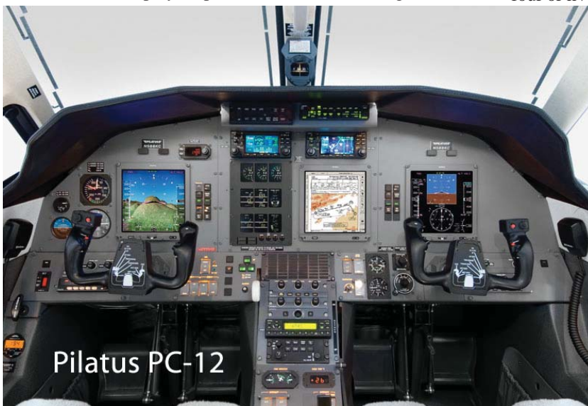
Universal Avionics’ EFI-890R features three 8.9 inch high-definition LCD screens that display a variety of data, including flight, terrain and electronic charts.
